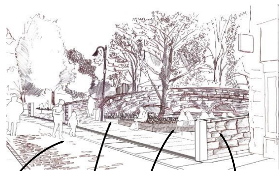
Streetscape paving adjusted to widen pedestrian pavement area, in order to accommodate fixed stone flood wall.
